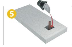
Cut away the formwork base to the requisite duct diameter using a hole saw/jig saw. Run the service duct/pipe through the penetration.
